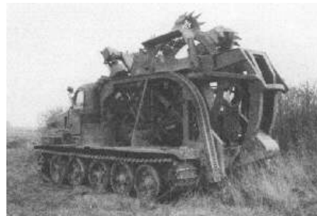
BTM ditching machine (8/4/0)
