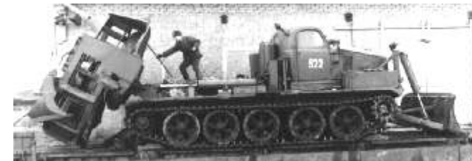
MDK-2 ditching machine (8/4/1)
